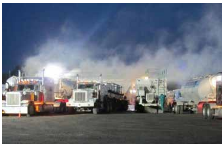
Silica dust clouds from delivery trucks loading into sand movers. Photo credit: NIOSH
